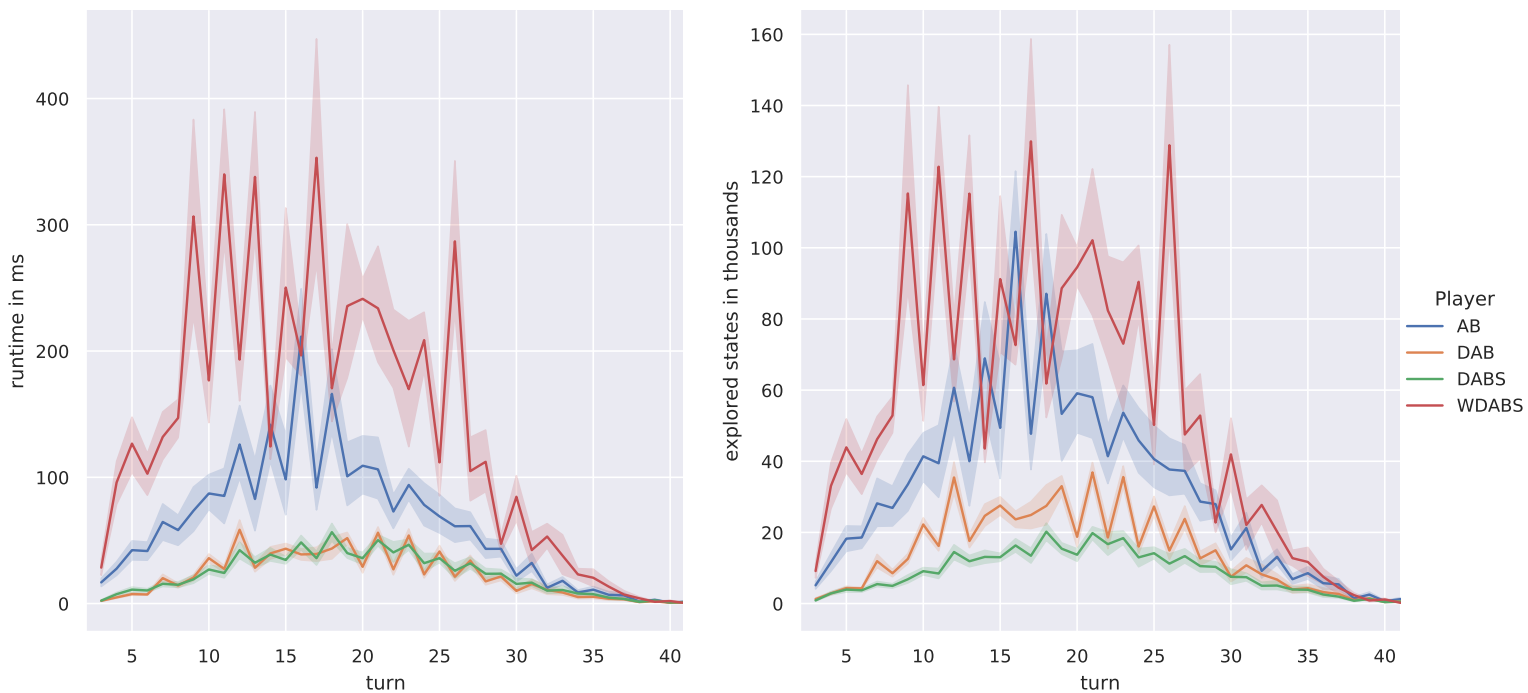
Figure 3.1: On an 8 \times 8 board AB, DAB and DABS search to depth 6; WDABS searches to layer 8 with 4 fields window padding.
