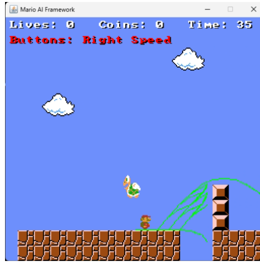
Figure 2.1: This screenshot illustrates the A* Agent of this thesis in a level. The green paths illustrate the traversed paths during the search of the previous frame. These were stored in the drawCoordinates array and subsequently displayed. It shows the agent exploring several paths that do not lead over the obstacle, the final path manages to overcome the obstacle and is subsequently chosen.
