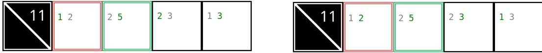
Figure 3.2: In this example, all values in the domain of the red-highlighted cell agree on the value 5 for the green-highlighted cell, this means every value assigned to the red cell forces the green cell to be assigned the value 5 after applying SIMPLIFY.
