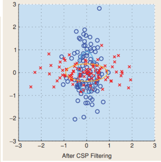
Fig. 2.9: After CSP filtering, the variance along the horizontal axis is maximized for the red class and minimized for the blue class, whereas along the vertical axis, the situation is reversed, demonstrating the CSP's efficacy in enhancing class separability..
