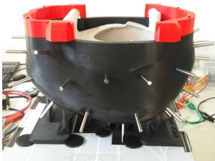
Fig. 1: Complete phantom with tank, skull, electrodes and support to hold the skull in place.
